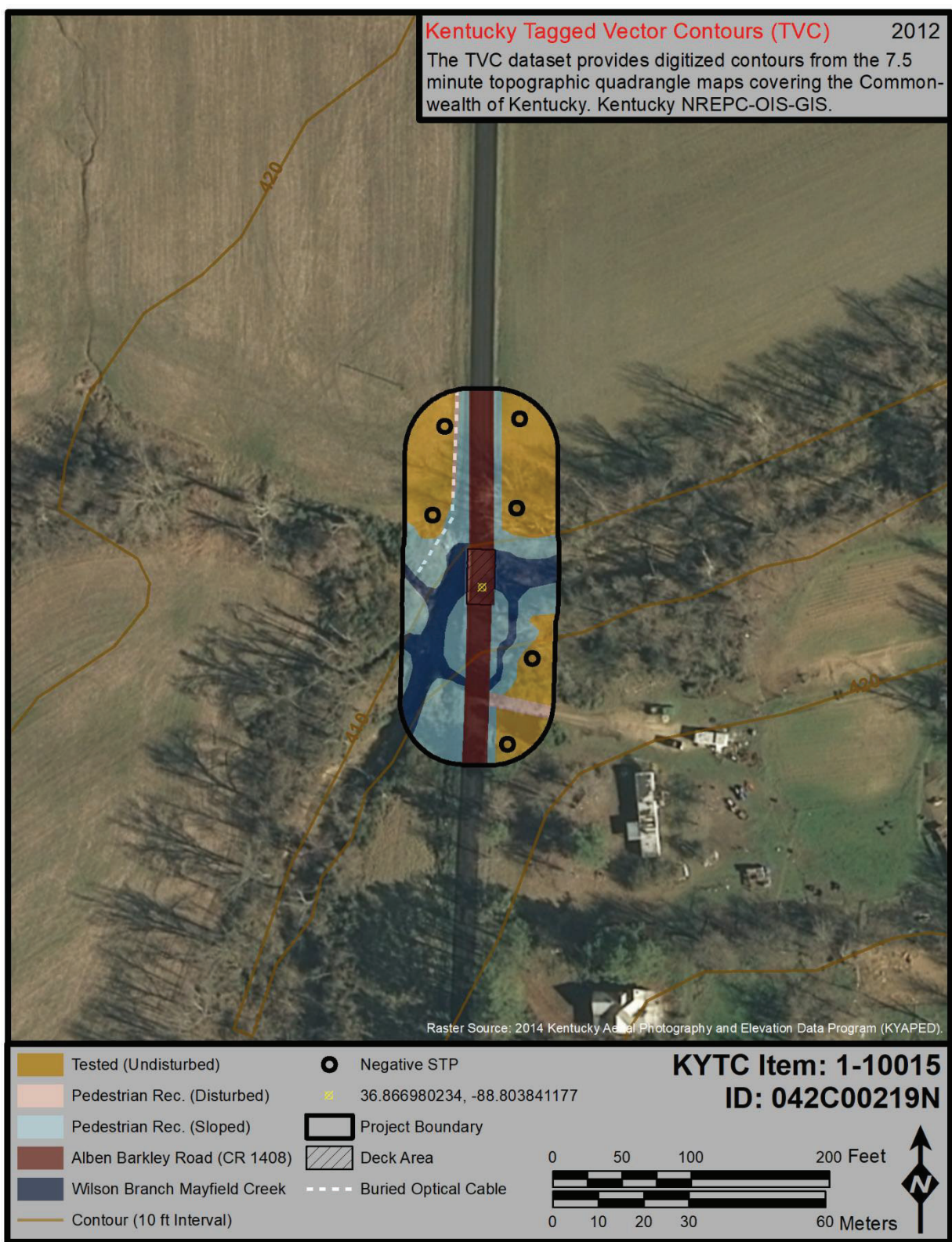
Figure 48. Bridge 042C00219N (Item No. 1-10015) showing project area conditions and excavated test locations on aerial map.
